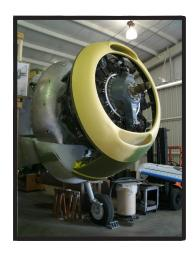
Sean and crew have installed the nose cowl, baffles, cowl flaps. These parts take quite a beating and it became obvious that all the shock mounts as well as the bearings need to be replaced and some sheet metal will need to be repaired.
