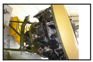
The firewall is painted, the oil tank has been installed. The engine is in place along with the oil cooler and is awaiting the crew to start hooking up the hoses and controls.
